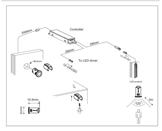
Technical Data Voltage: DC 12V~24V Max Load: 5A DetectionArea: 3meters DetectionAngle: Max. 120° Time-delay: 35 seconds Protection Class: IP20
