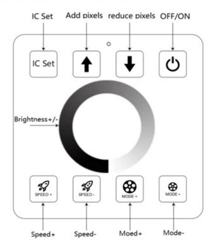
IC Set point setting: short press IC Set to enter the adjustment point setting, press the up button to increase the point, press to the down button to decrease the point, short press to adjust 1 IC, long press to quickly adjust, and press the shutdown button to save after adjustment. The default factory is 80 pixels, and the maximum can be adjusted to 2048 pixels. Ring: Brightness plus or minus.
