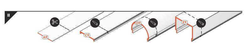
Note! The length of the cover is equal to the length of the profile.
