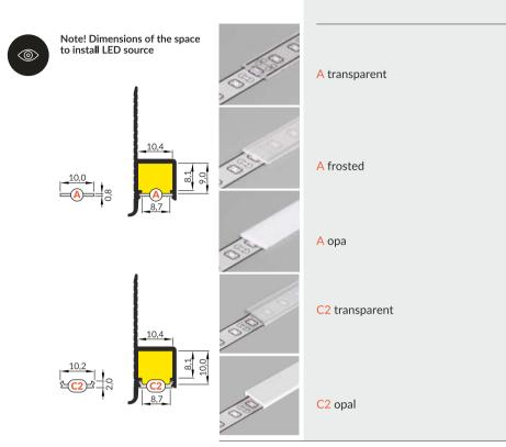
The standard cover length tolerance is  $\pm 20$  mm.
