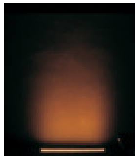
30° Front View Distance to the wall is 200mm Graze height on the wall is 3000mm
