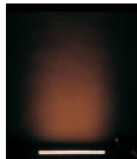
30° Front View Distance to the wall is 300mm Graze height on the wall is 3800mm
