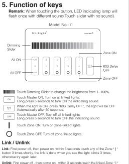
Unlink: First power off , then power on , within 3 seconds touch the linked Zone ' | ' button or the Master ' | ' button 5 times shortly , the unlink is done when you see the light blinks 9 times, otherwise try again later.
