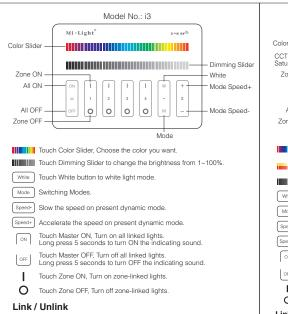
Link: First power off, then power on, within 3 seconds touch any of the Zone '  $\mid$  ' button 1 time shortly, the link is done when you see the light blinks 3 times, otherwise try again later.
