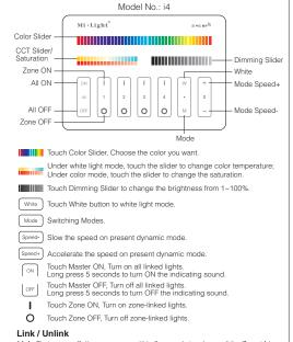
$\label{eq:Link: First power off, then power on, within 3 seconds touch any of the Zone ' | ' button 3 times shortly, the link is done when you see the light blinks 3 times with green color, otherwise try again later.$
