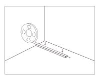
The specific glowing effect can be adjusted according to the needs of the application. After the installation, connect the light to the low-voltage driver and energize it.
