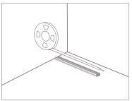
Put the light into the aluminum profile, and press the light down along the profile to ensure the light is tightly stuck into it. Then
