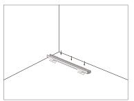
Put the light into the aluminum profile, and press the light down along the profile to ensure the light is tightly stuck into it. Then fasten the profile on the rotating brackets (according to the glowing angle requirements, the rotating bracket can be adjusted).
