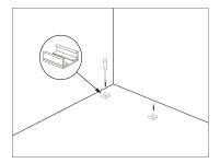
Remove the stainless steel mounting clips and screws from the packing box, and use a screwdriver to install these clips where needed.
