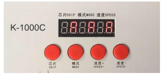
3. After finished address code, press "CHIP" first and at the same time press "MODE" button, switch to playback mode, switch the chip to Chip: 10, this is the DMX512 standard agreement 250Kbps playback mode. At this time, press MODE button and SPEED button can separately switch playback mode and adjust speed, as below:
