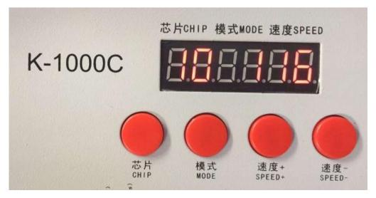
Special Remarks: Derived program after set one-key coding in the software, long press MODE for 5 seconds can write code to the lights directly, this function is very convenient and practical. Welcome to consult our engineer or salesman to learn the detailed operation method.
