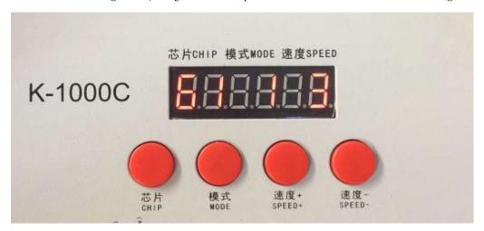
NOTE:61 means UCS512A or B coding mode; 62 means WS2821 coding mode; 63 means SM DMX512AP; 64 means UCS512-C; Ch.: 03 means the coding channel is 3 channels
