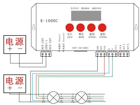
Single signal wiring diagram:
