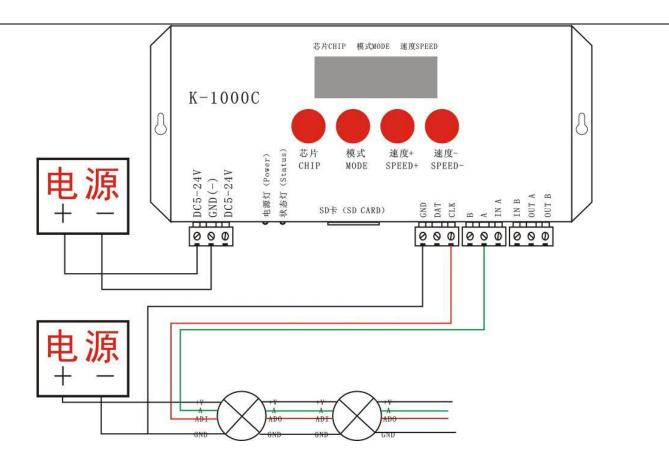
1. Like the above diagram, wired the line and start the controller, press "CHIP" and "MODE" at the same time switch to coding mode, adjust to Chip: 61 that is UCS512A or B coding mode, as below:
